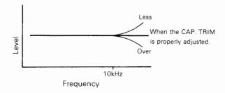
Select the optimum load capacitance for your MM cartridge of the turntable connected to the PHONO MM jacks by referring to the table below.
